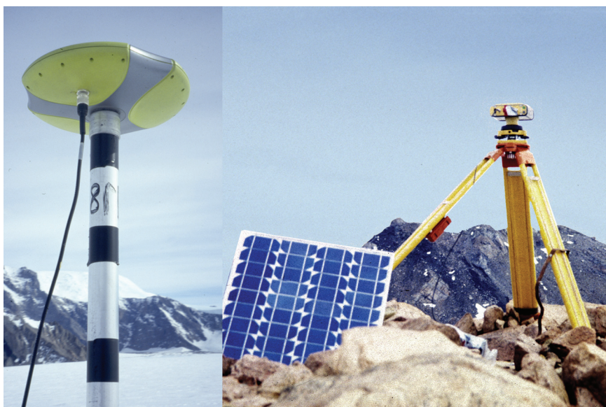
Fig. 5. JPS Legacy E antenna on a stake (left) and the base station with a Hiper antenna-receiver placed on a fixed point on the bedrock (right). The base station was connected to a solar panel. Photos: FINNARP/Anna Sinisalo.
