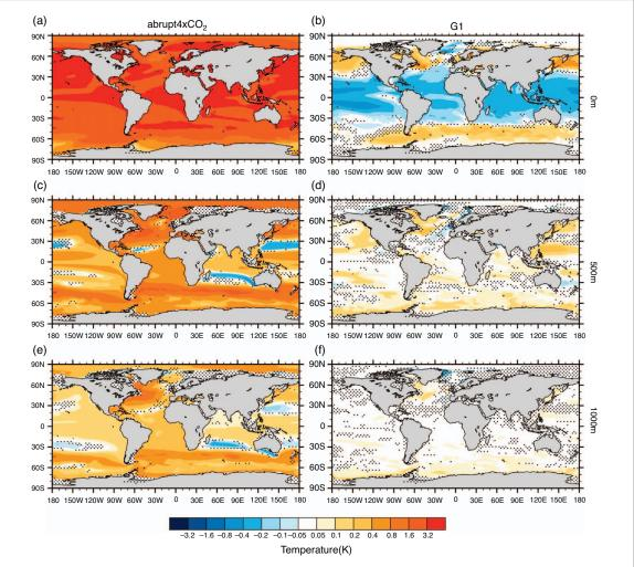
Figure 1. Left column: Ocean temperature anomalies of  $abrupt4 \times CO_2$  (11–50 yr) relative to piControl. Right column: Ocean temperature anomalies of GI (11–50 yr) relative to piControl. The different rows are for different depths in the ocean. Stippling indicates where fewer than 5 out of 7 agree on the sign of the change.
