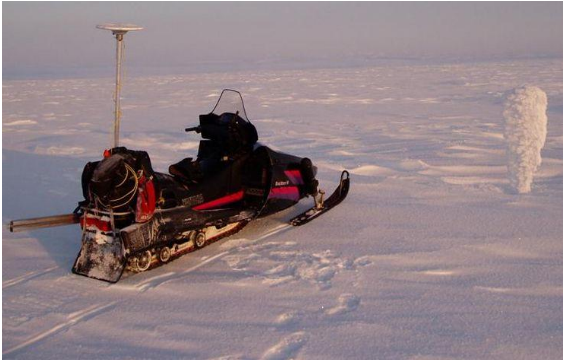
Measuring position of massbalance stakes and making surface leveling. Sometimes the aluminum pipes we drilled 2007 was hard to find, this one made a nice ice rime statue. Photo: Veijo Pohjola.
