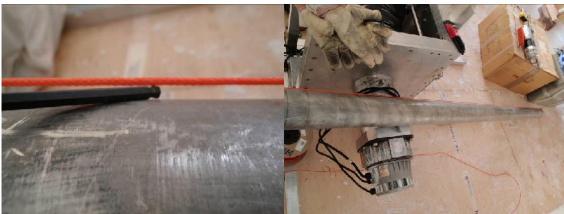
Bent outer barrel. (Photos: Mike Gerasimoff)
