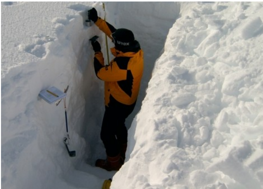
Christoph Schneider doing snow density measurements in snow pit on Ahlmann Summit
